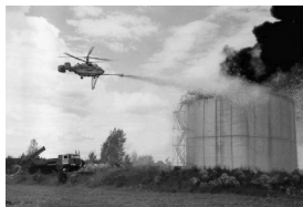
Pic. 2. Fire extinguishing with defoaming agents at oil storage with water dispersing guns.
