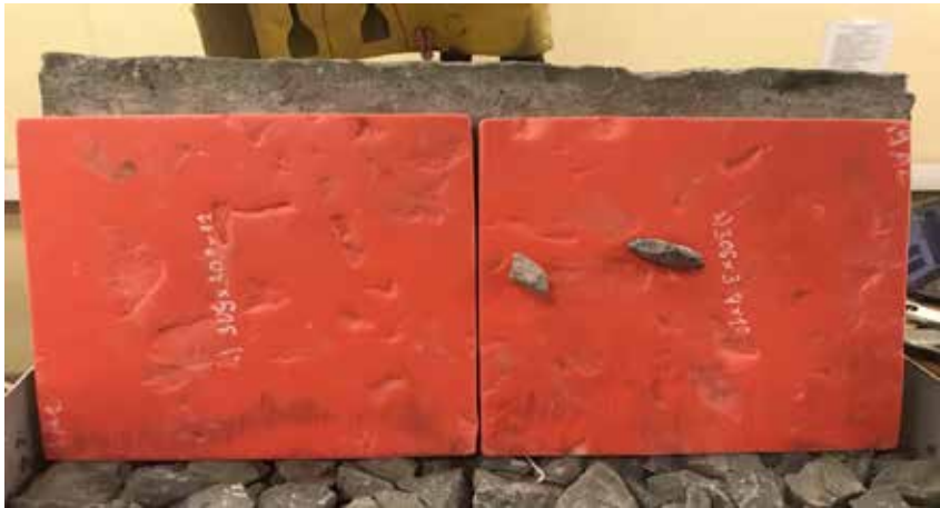
Pic. 5. Appearance of intermediate-type USP after testing [photo taken by the authors].
