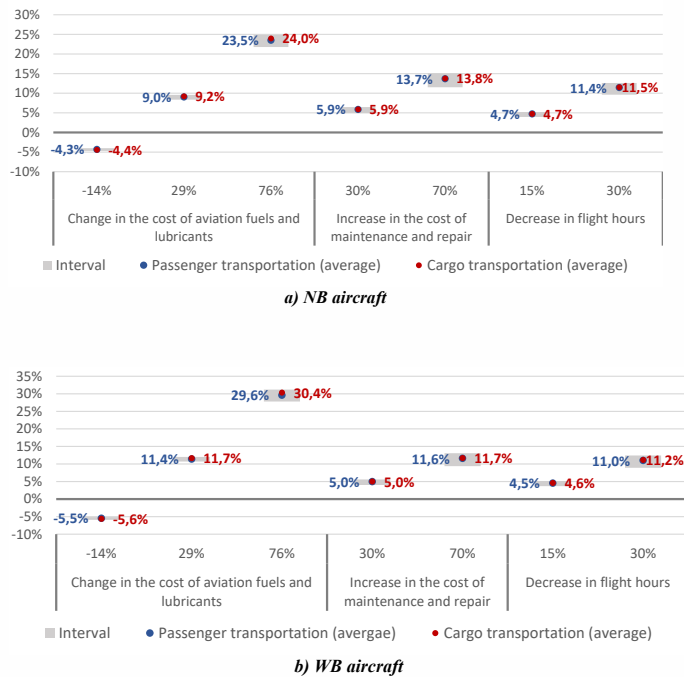
Pic. 6. Change in direct operating costs with varying factors [performed by the authors].
