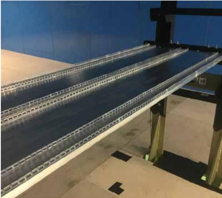
Pic. 11. Model of the span structure [performed by O. I. Poddaeva, P. S. Churin, A. N. Fedosova].
