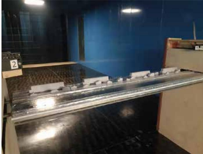
Pic. 12. Model of the bridge span structure (car traffic) [performed by O. I. Poddaeva, P. S. Churin, A. N. Fedosova].
