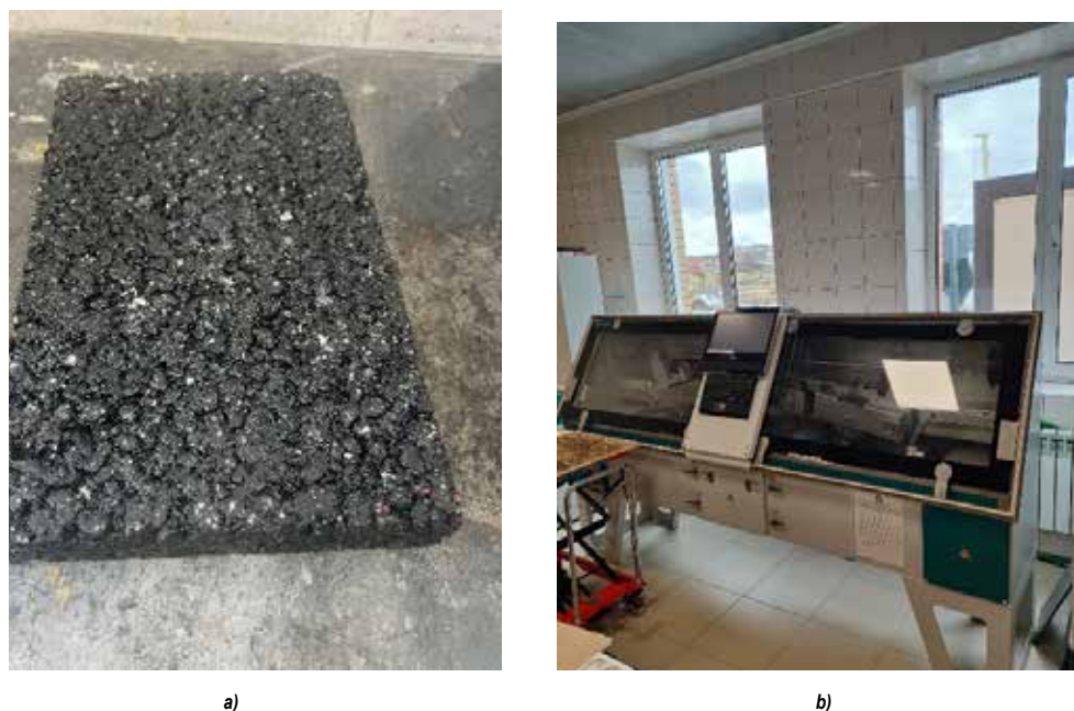
Pic. 4. Preparation of control sample slabs (a) with testing on a load wheel rolling tester (b) [performed by the authors].
