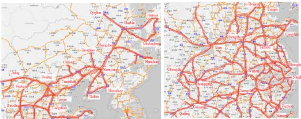
Pic. 8. Topology of the HSR network of northern China (left) and central China (right) [performed by the authors using an open-source topographical survey at the openrailwaymap].
