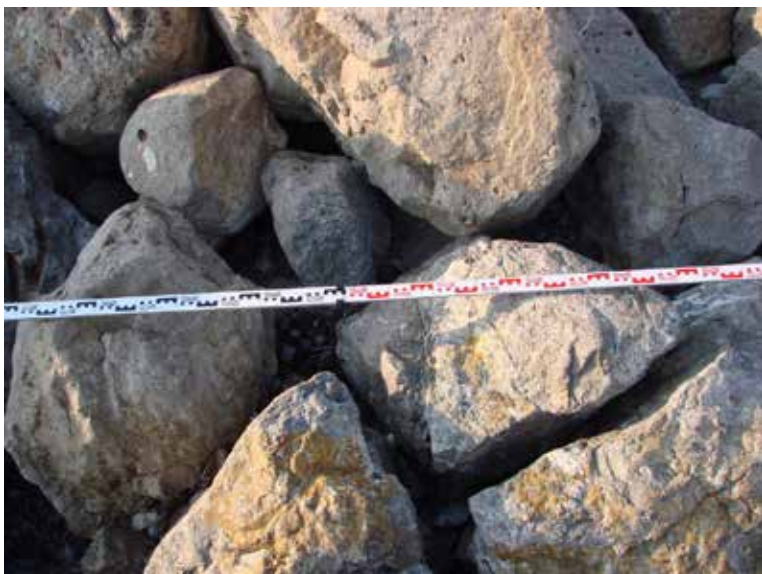
Pic. 4. Assessment of stone size in stone spur dikes [photo by the author, 20.07.2007].
