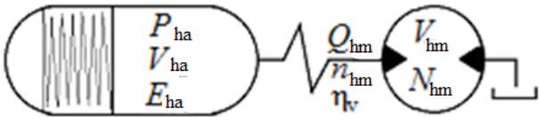
Pic. 2. Calculation scheme of the hydraulic drive of the plate feeder.
