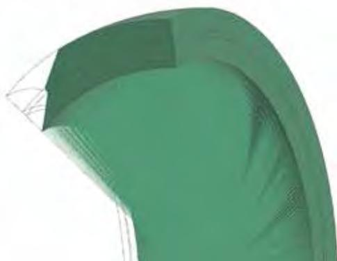
Pic. 6. The shape of the hinge with equal elasticity of rubber layers according to the simulation results [obtained by the authors].
