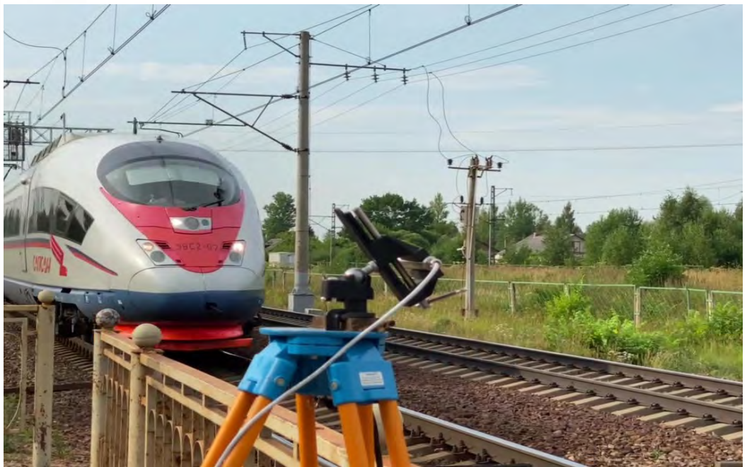
Pic. 10. The process of measuring the aerodynamic impact from the Sapsan high-speed electric train [image made by the author].
