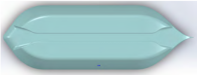
Pic. 8. Change in the geometry of the tail fairing in the models No. 3 and No. 4 [developed by the authors].
