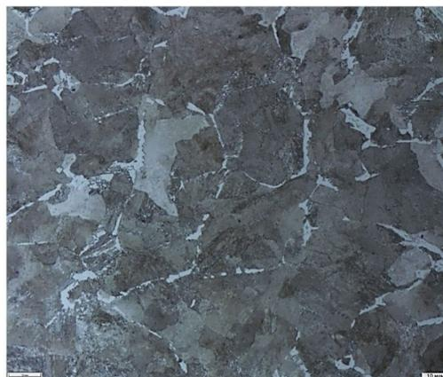
Pic. 1. Microstructure of main metal of wheel steel of type 2, x1000 [developed by the authors].
