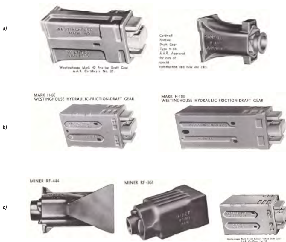
Pic. 3. Types of draft gear used on American railways: a) friction; b) hydraulic-friction; c) rubber friction [16].
