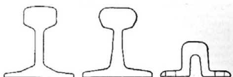
Pic. 6. Wide-sole rail used on railways, respectively, on New South Wales Railway, Midland Great Western Railway, Great Western Railway. [Electronic resource]: https://www.1902encyclopedia.com/RAI/railway-27.html . Last accessed 11.06.2021.
