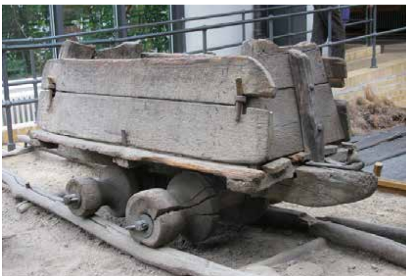
Pic. 8. Wooden trolley on wooden guides (beds) with wheels with flanges. (History of railway transport. [Electronic resource]: https://ru.wikipedia.org/wiki/История_железнодорожного_транспорта . Last accessed 11.06.2021).
