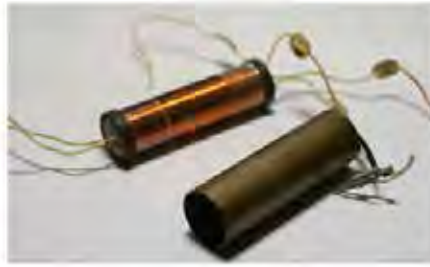
Pic. 1. Structure of a fluxgate sensor: H – fluxgate sensor's excitation field, H_0 – measured magnetic field (compiled by the authors).
