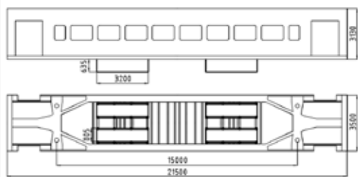
Pic. 1. Structural diagram of an electric train wagon body (the author's diagram).
