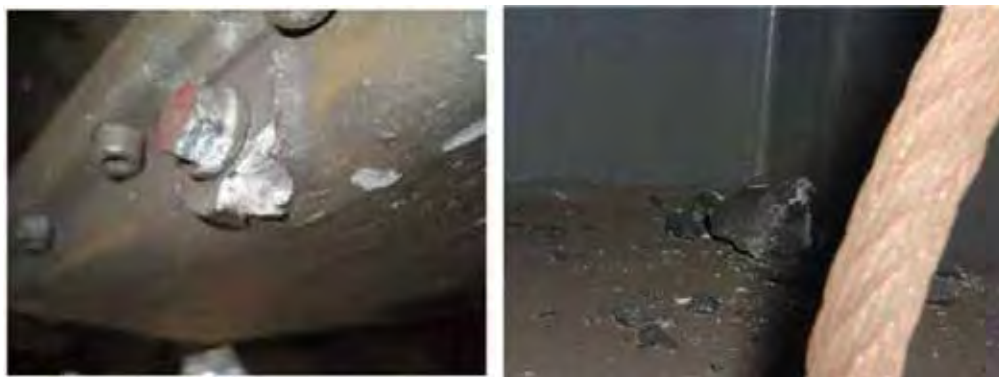
Pic. 1. Damage to the car body from impacts of crushed stone particles [6].
