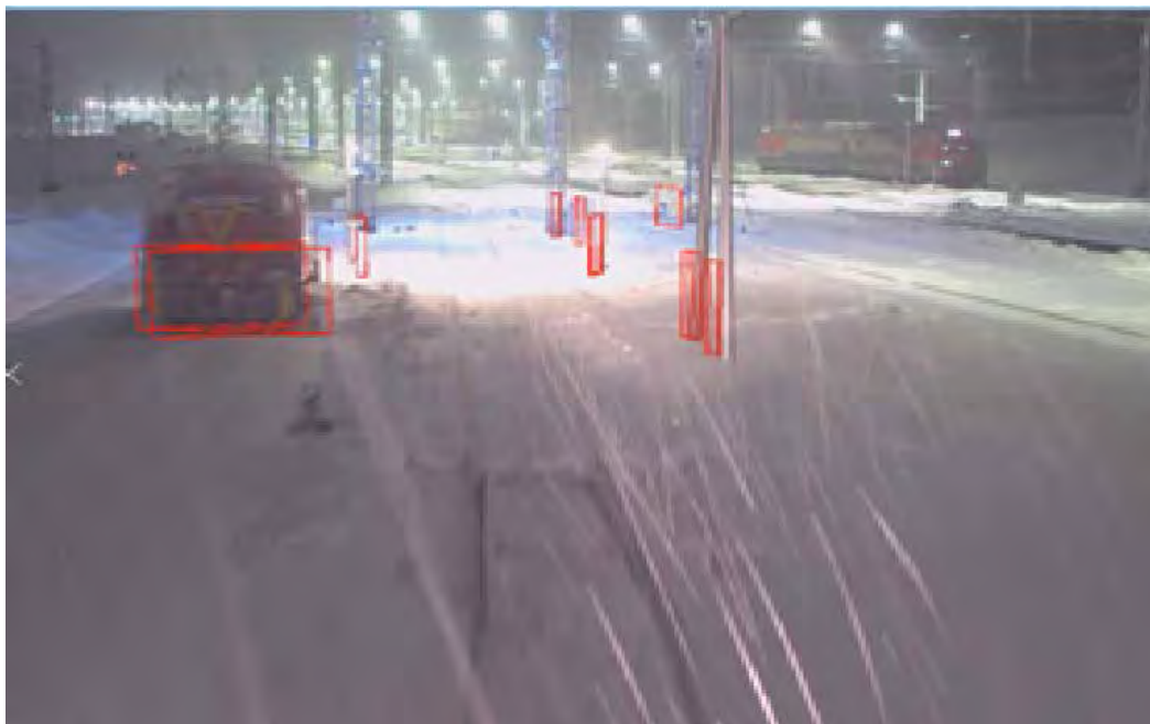
Pic. 4. Information situation of poor visibility requiring a probabilistic assessment. [Electronic resource]: https://railvision.io/main-line-solution/ .
