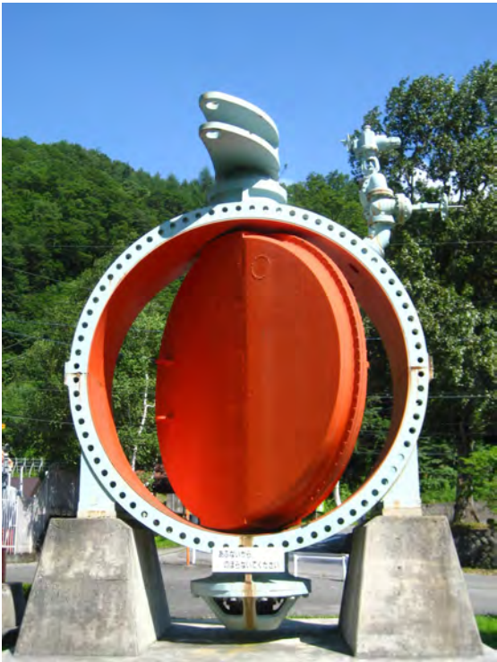
Pic. 4. A large shutter with a flat-blade disc used at a hydropower plant in Japan [1; 2]. [Electronic resource]: https://commons.wikimedia.org/wiki/File:Yagisawa_power_station_inlet_valve.jpg?uselang=en . Last accessed 22.07.2019.
