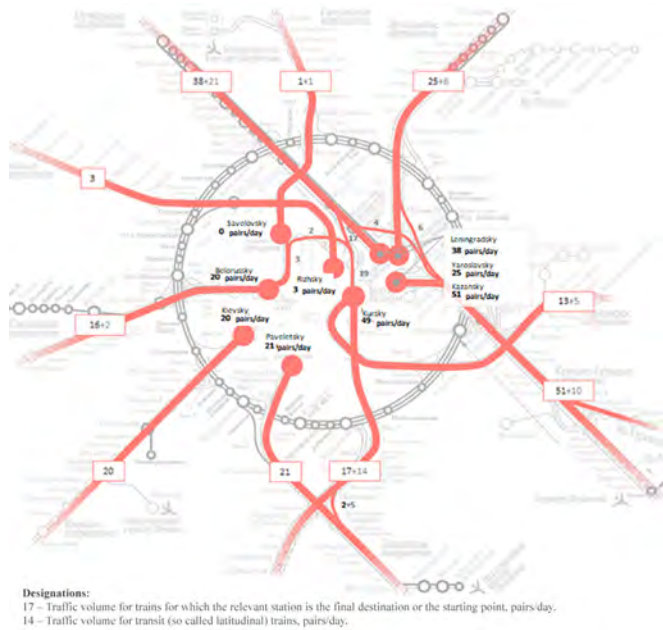
Pic: 1. The existing scheme of long-distance passenger trains traffic within Moscow railway junction (compiled by the authors).
