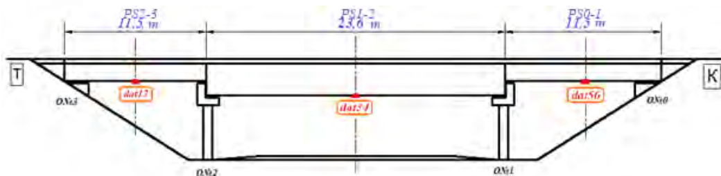
Pic. 1. Layout of resistance strain gages on span structures of railway reinforced concrete overpass, at 97 km PK5+20, PS0–1, PS1–2, PS2–3 – span structures of the overpass; dat 1, 2, 3, 4, 5, 6 – resistance strain gages FLM-60–11; O No. 1, O No. 2 – frame, two-rack intermediate supports; O No. 0, O No. 3 – foundations of talus type (authors' picture).
