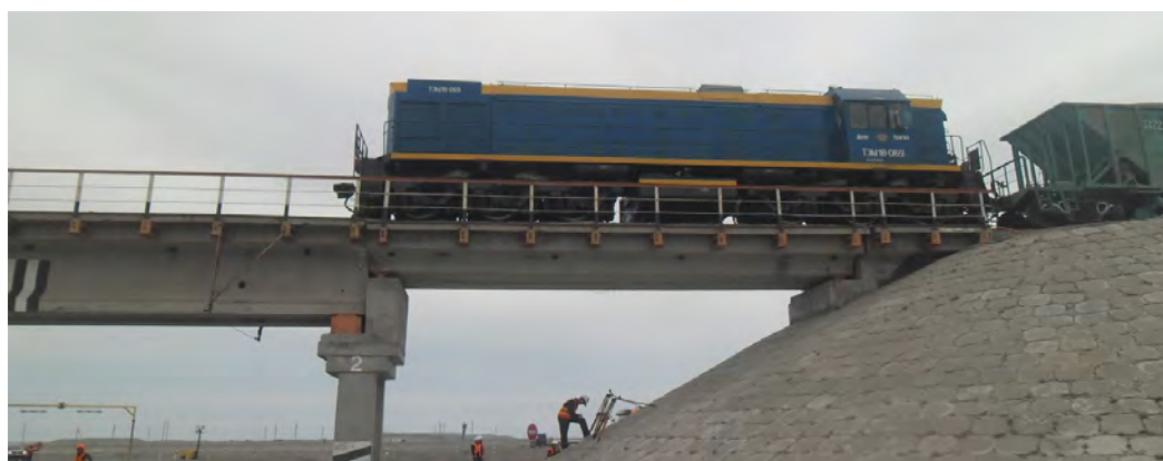
Pic. 3. Photo of installation of the train «locomotive-car» on a span structure 0–1 (load C1) (authors' photo).
