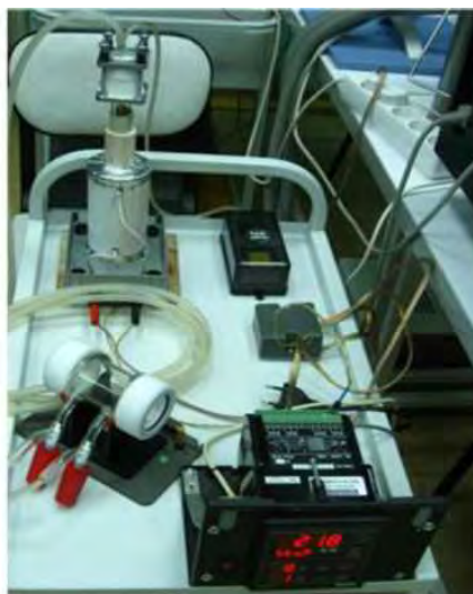
Pic. 4. Temperature-controlled attachment for the study of gaseous products from an insulating material with a calibration cuvette.
