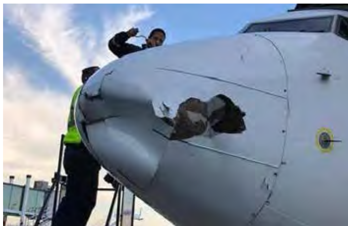
Pic. 5. Airliner damaged following the collision with UAV [20].
