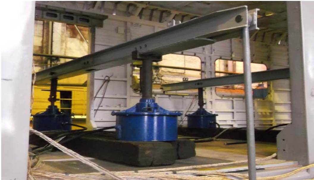
Pic. 3. The application of the vertical load on the metal work of the car body with pneumatic equipment.
