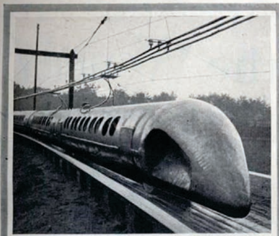
Above, note the fishlike snout of the new Russian monorail that runs in a trough. At right, the strange train in action. In circle, M. I. Yarmanchuk, the inventor
