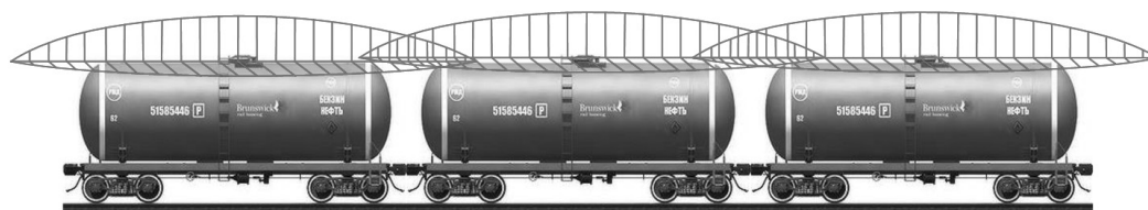
Pic. 2. Scheme of overlapping adjacent explosion hazardous areas.
