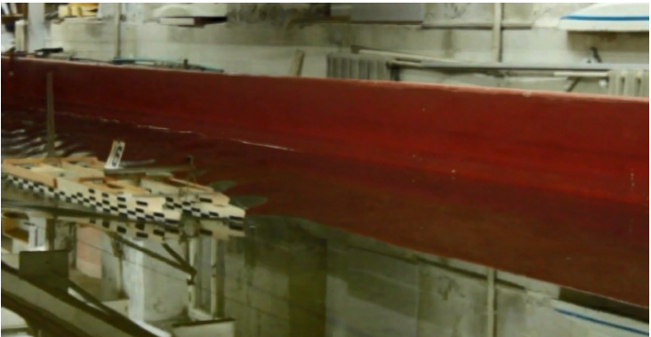
Pic. 3. Test of a catamaran model.
