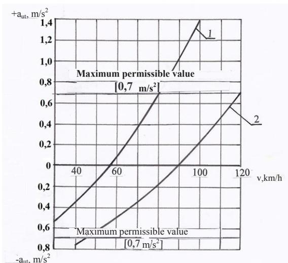
**Pic. 1. Dependence of unextinguished transverse acceleration on the speed of tank movement on curved sections of the track: 1 – curve with radius of 350 m; 2 – curve with radius of 650 m.**
