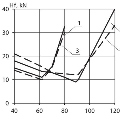
**Pic. 4.** Dependence of the constant component of frame force on climbing wheel set on the speed of movement of tanks on the railway track curves: 1 and 2 – four-axle tank in curves with a radius of 350 and 650 m, 3 and 4 – eight-axle tank in curves of the same radii.
