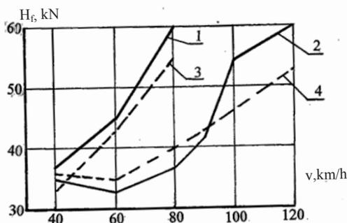
**Pic. 3.** The maximum values of the total frame force on the climbing wheel set at movement in curves of the rail track: 1 and 2 – four-axle tank in curves with a radius of 350 and 650 m, 3 and 4 – eight-axle tank in the curve of the same radius.
