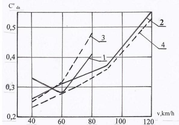
identical. However, theoretical calculations indicate that for the same values of relative friction force of friction dampers and static deflection of spring suspension of four-axle and eight-axle tank cars coefficient of dynamic addition of vertical forces in the latter is 20–25% less than that of four-axle one due to more (twice more) wheel sets in the bogie of the eight-axle tank car.
