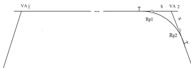
Pic. 3. Fixing tangent lines with reference marks.
