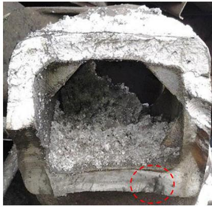
**Objective.** The objective of the author is to consider situation with cast parts of bogie's side frame, namely fractures and rejection criteria.
