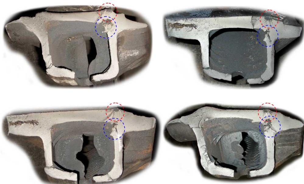
**Pic. 6. Internal defects in fractures of side frames of the same series.**
