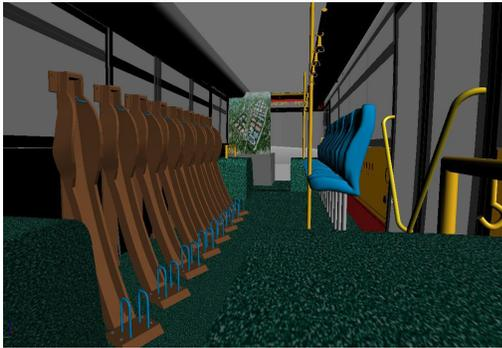
Pic. 4. Racks for mounting a bicycle in bicycle-bus.
