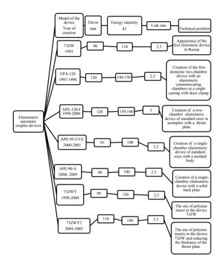
Pic. 1. Development chronology of elastomeric draft gears of the automatic coupler.
