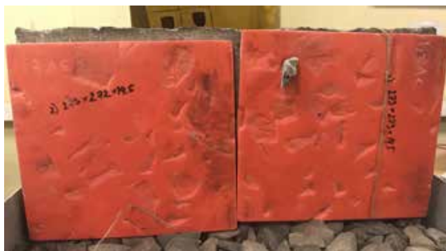
Pic. 4. Appearance of soft-type USP after testing [photo taken by the authors].
