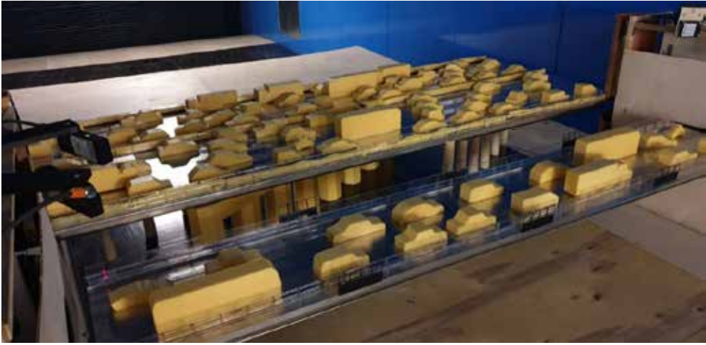
Pic. 8. Scheme of the experiment to assess the number and location of vehicles on the span structure for its aerodynamic stability [performed by O. I. Poddaeva, P. S. Churin, A. N. Fedosova].
