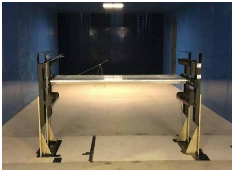
Pic. 4. Installation for testing a model of a bridge crossing in a wind tunnel [performed by O. I. Poddaeva, P. S. Churin, A. N. Fedosova].
