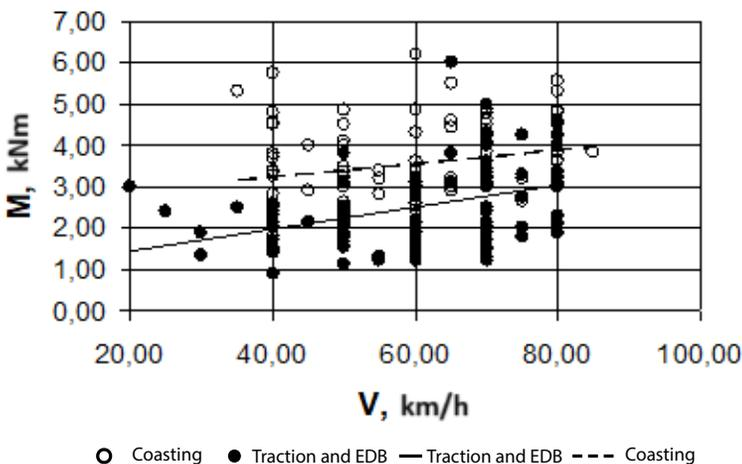
*Pic. 12. Maximum dynamic torque on the shaft of the axle gearbox of the 2TE121-011 diesel locomotive, Vorkuta – Sosnogorsk section, in different driving modes [according to data obtained by O. V. Izmerov].*
