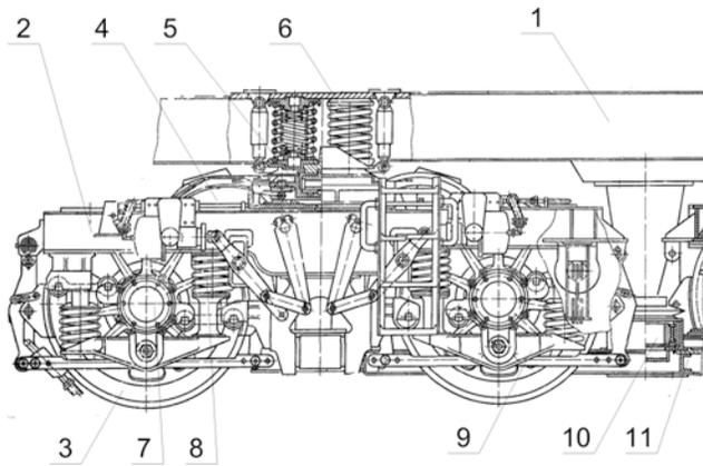
**Pic. 2. Bogie of TE136 diesel locomotive: 1 – body frame; 2 – bogie frame; 3 – wheelset; 4 – TEM; 5 – support and return devices; 6 – second stage of spring suspension; 7 – axle box; 8 – axle box stage of spring suspension; 9 – balance beam; 10 – kingpin assembly; 11 – low-mounted frame [9].**
