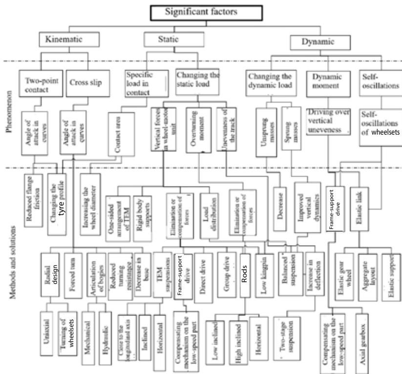
Pic. 1. Classification of methods for improving adhesion properties by changing the design of the undercarriage, proposed by the authors of the article.
