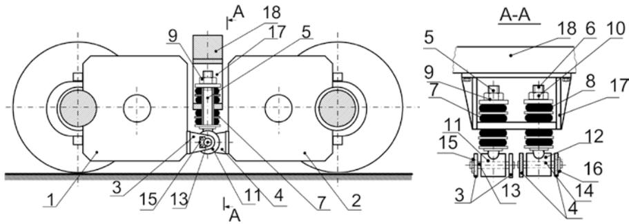
**Pic. 5.** Arrangement of TEM suspensions on an axis passing through the bogie's centre of gravity. 1, 2 – TEMs; 3, 4 – brackets; 5, 6 – rods; 7, 8 – rubber washers; 9, 10 – nuts; 11, 12 – hinges; 13, 14 – shafts; 15, 16 – strips; 17 – crossbeam; 18 – bogie frame [10].
