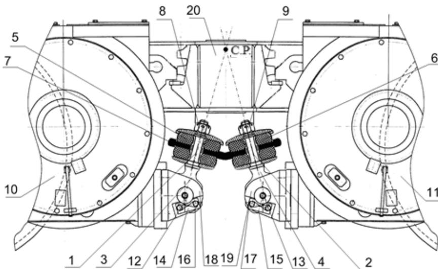
**Pic. 6.** Device for fastening the locomotive traction motor to the bogie frame: 1, 2 – suspensions; 3, 4 – hinges; 5, 6 – sets of flat elastic elements; 7 – crossbeam; 8, 9 – nuts; 10, 11 – traction electric motors; 12, 13 – shafts; 14, 15 – locking strips; 16, 17 – bolts; 18, 19 – brackets; 20 – bogie centre of gravity [11].
