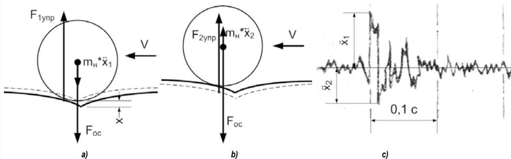
**Pic. 7. Changes in axial load during oscillations of unsprung masses:**
