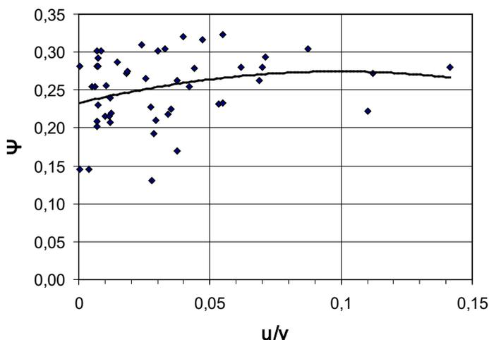
*Pic. 13. Empirical dependence of the axle adhesion coefficient  $\psi$  of 2TE121–003B diesel locomotive on the relative slip speed  $u/v$  in case of development of self-oscillations of the wheelset [according to data obtained by O. V. Izmerov].*
