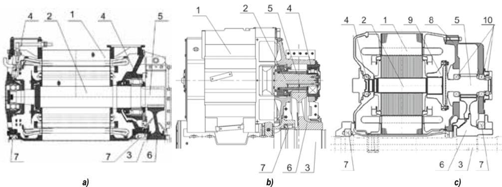
**Pic. 10.** Axle-support drive with rigid gear transmission: a) TE33a diesel locomotive; b) BKG-1 electric locomotive; c) 2EV-120 electric locomotive; 1 – TEM; 2 – TEM shaft; 3 – wheelset axle; 4 – rotor bearing; 5 – small gear wheel; 6 – large gear wheel; 7 – axle bearing; 8 – gearbox housing; 9 – diaphragm coupling; 10 – gearbox bearings [29].
