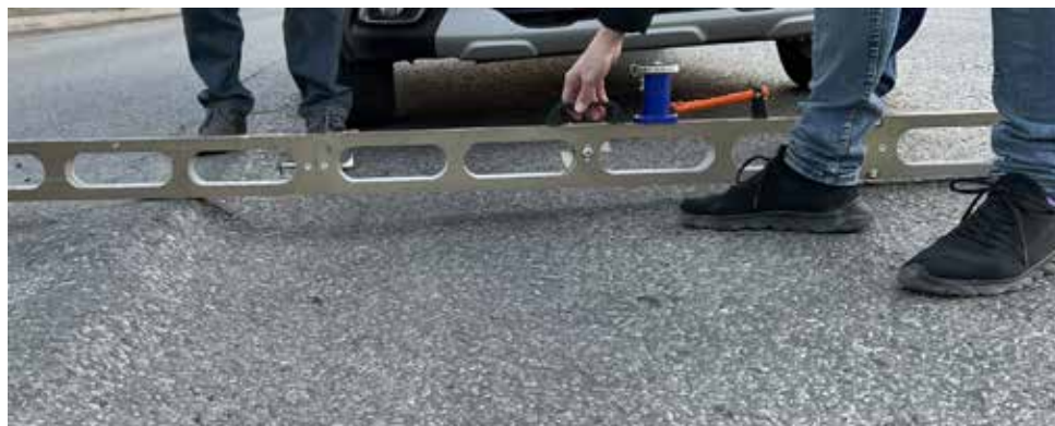
Pic. 1. Ridge of the uplift of the asphalt concrete pavement with a surface plastic rut [photos by the authors].
