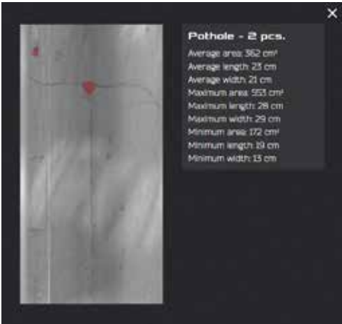
Pic. 3. The result of the algorithm's operation regarding the «Pothole» class [developed by the authors].
