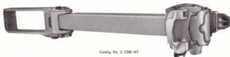
Pic. 1. AAR Alternate Standard Controlled Slack Coupler with Drawbar [USA Car and Locomotive Cyclopedic of American Practice. 2 nd edition by C. L. Combes (Editor). New York, Simmons-Boardman Publication Corporation, 1970, 1074 p. ISBN-10 1122559348, ISBN-13 978-1122559348].
