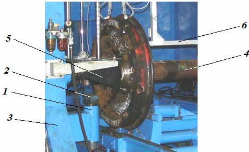
Pic. 4. Fragment of a device for moving wheelsets as part of the system 3 for measuring geometric parameters: 1 – mechanism for vertical movement of a wheelset to the measurement position (hydraulic cylinder), 2 – support with pads, 3 – installation stand for measuring geometric parameters, 4 – wheelset in measurement positions, 5 – block for measuring the diameters of the axle journal, 6 – block for measuring the diameters of the wheelset axle [14].
