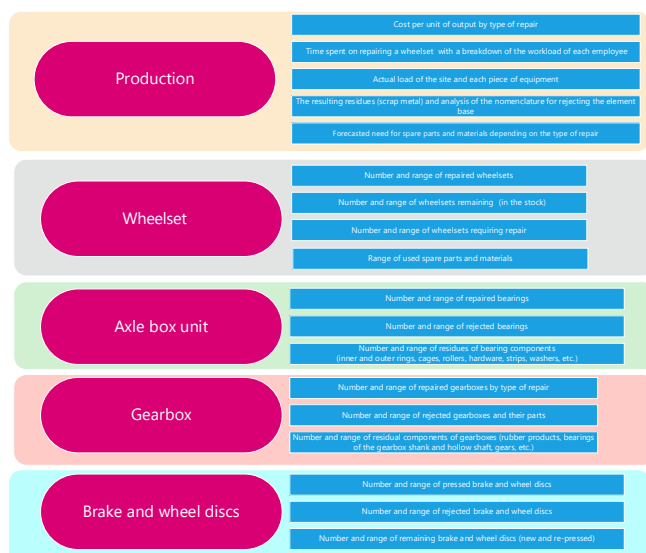
Pic. 4. Structure of digital indicators of operation of the wheel-roller repair workshop [performed by the authors].
