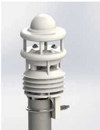
Pic. 9. Sensor for recording basic meteorological parameters.
