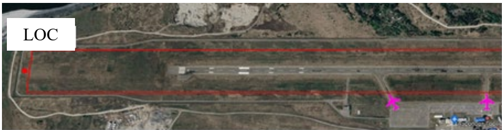
Pic. 8. Positioning of aircraft with dimensions corresponding to the Boeing-737 near the border of the LOC critical area.
