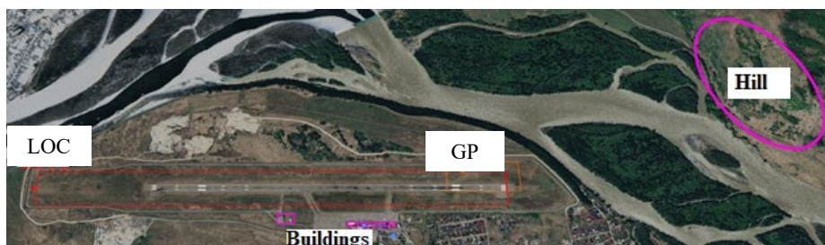
Pic. 5. Satellite image of the runway of Gorno-Altai aerodrome indicating the GP and LOC critical areas, as well as reflecting objects (a hill and buildings).
