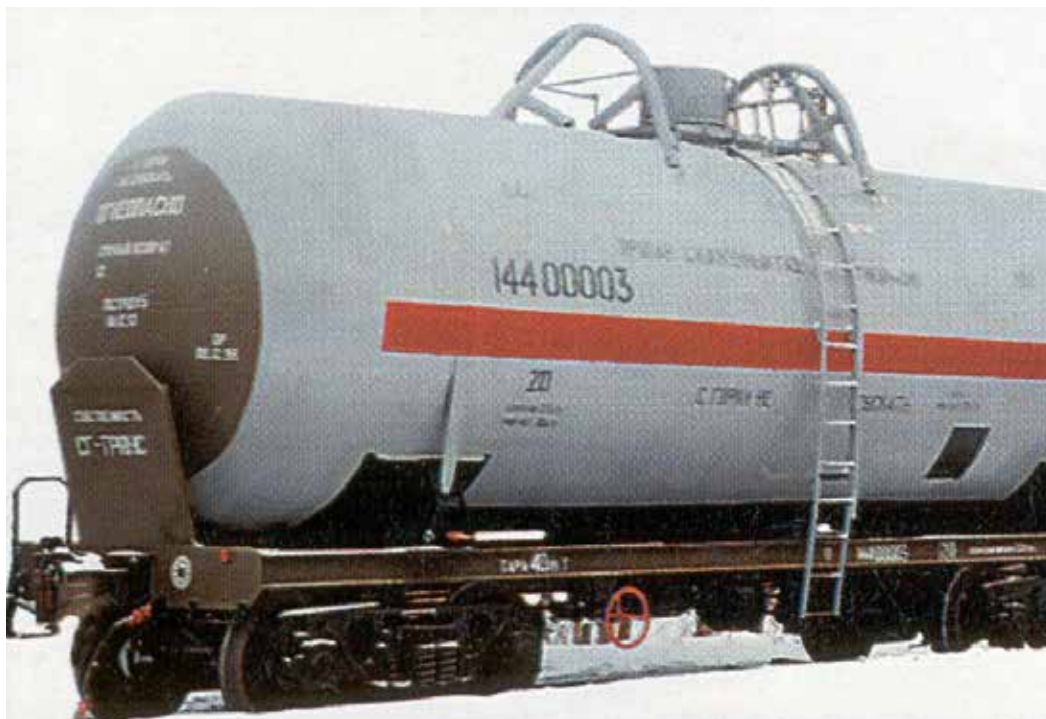
Pic. 1. A serial tank car for liquefied hydrocarbon gases with technical means of protecting the boiler in emergency conditions (photo of the Department of Wagons and Wagon Facilities of RUT).
