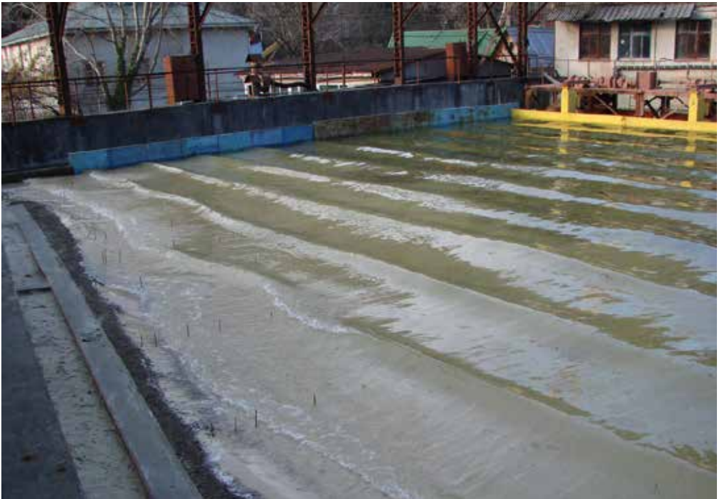
Pic. 2. Laboratory studies of structures for protection of linear structures (railway roadbed) in a wave basin [performed by the author].
