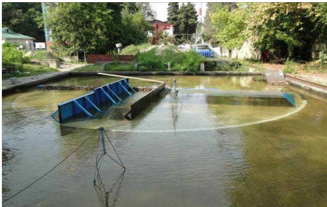
Pic. 4. A wave basin with a turntable for laboratory studies with various angles of wave approach to structures [performed by the author].
