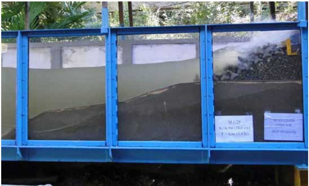
Pic. 3. Laboratory studies of a sloping wave-damping structure made of shape arrays (tetrapods) with a frontal approach of waves in a wave tank [performed by the author].
