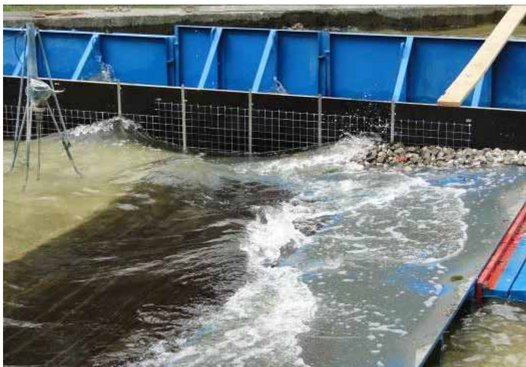
Pic. 5. Laboratory studies of a sloping wave-damping structure made of stone in a wave basin [performed by the author].
