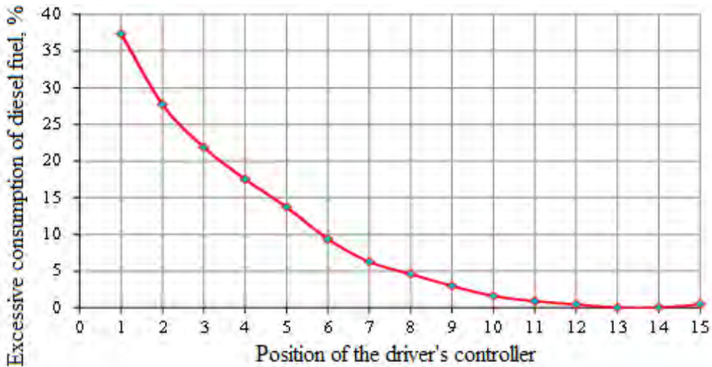
Pic. 1. Excessive consumption of diesel fuel depending on the position of the driver's controller [performed by the authors].
