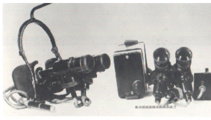
Pic. 4. Night vision devices of SDB-1, manufactured by Experimental Electromechanical Plant of VEI. 1942-1945 years.
