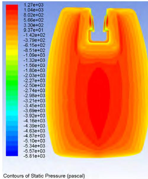
*Pic. 12. Pressure distribution over the frontal surface of the model No. 4 [developed by the authors].*
