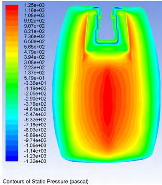
*Pic. 11. Pressure distribution over the frontal surface of the model No. 3 [developed by the authors].*
