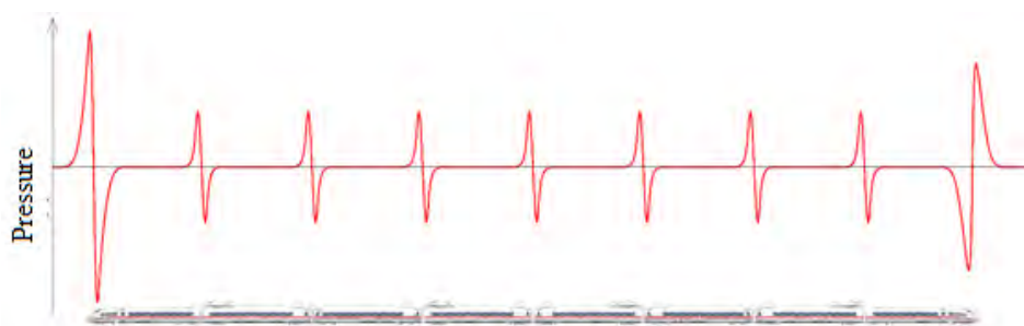
Pic. 1. Principal graph of the change in the magnitude of air pressure along a high-speed train [developed by the author].
