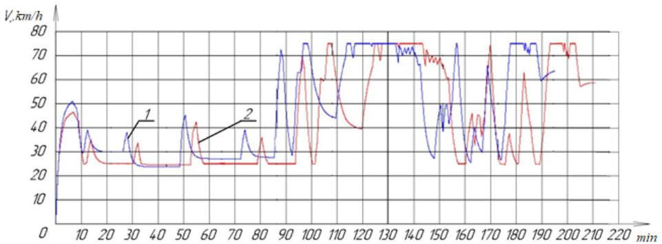
Pic. 5. Change in train speed when moving along a III class track profile depending on the travel time  $V = f(t)$ :
