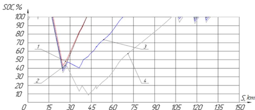
Pic. 7. Discharge curves of the traction battery TES of locomotives with a hybrid power plant: 1 – a train with a weight of 4600 tons and TES with 1 cell of the traction battery; 2 – a train with a weight of 4900 tons and TES with 6 cells of a traction battery; 3 – a train with a weight of 5250 tons and TES with 11 cells of a traction battery; 4 – a train with a weight of 5750 tons and TES with 18 cells of a traction battery [performed by the authors].
