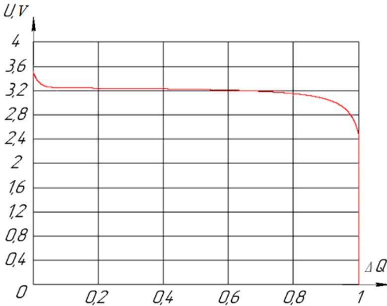
Pic. 4. Discharge characteristic of the simulated battery  $U = f(\Delta Q)$  [performed by the authors].
