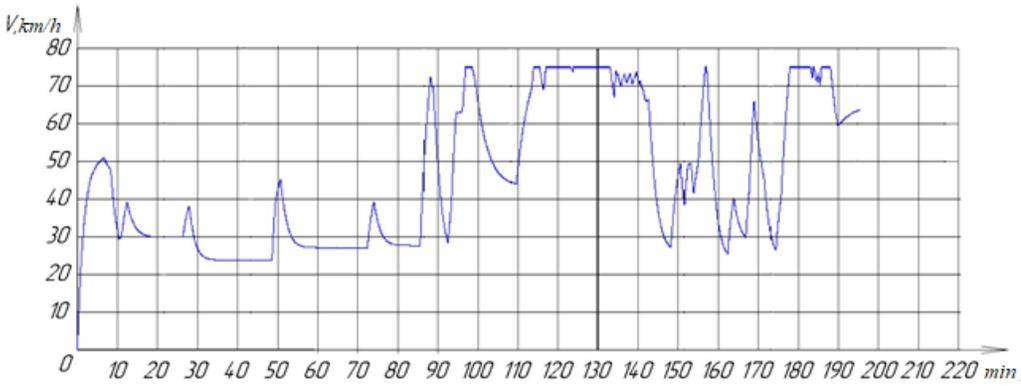
Pic. 2. Change in the speed of a diesel locomotive with a standard power plant and the train of the calculated weight when moving along a class III track profile depending on the travel time  $V = f(t)$  [performed by the authors].
