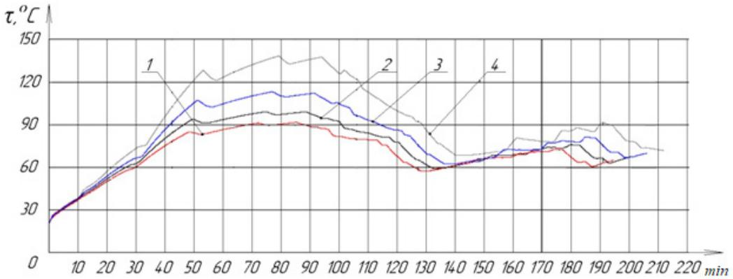
Pic. 6. Curves of the temperature rise of the armature winding of the traction electric motors of a hybrid diesel locomotive when moving with trains of increased weight:
