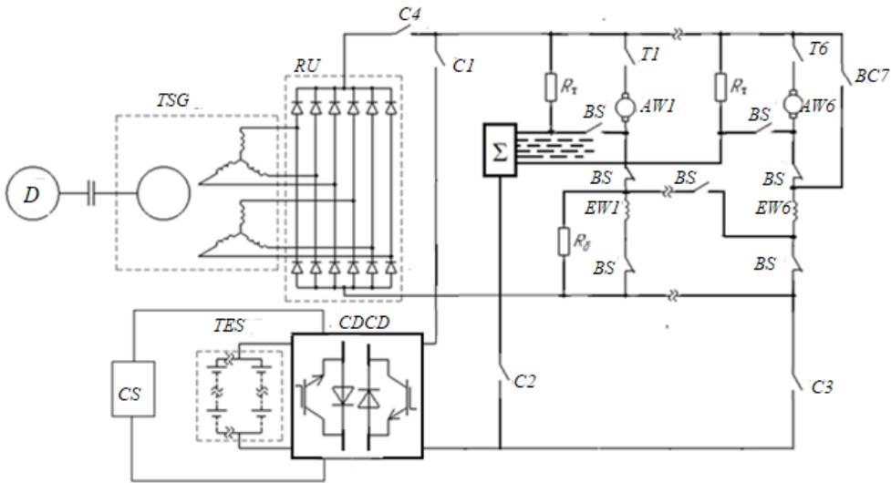
**Pic. 1. Traction electrical circuit of a hybrid diesel locomotive with AC-DC transmission, T1 – train contactor switch of TEM 1; T6 – train contactor switch of TEM 6; BC7- braking contactor; EW1 – excitation winding of TEM1; EW6 – excitation winding of TEM6; AW1 – armature winding of TEM1; AW6 – armature winding of TEM 6 [performed by the authors].**
