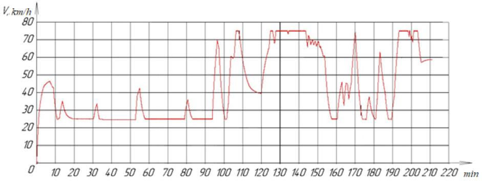
Pic. 3. Change in the speed of a diesel locomotive with a hybrid power plant when moving with a train of 5750 tons of weight along a III class track profile depending on the travel time  $V = f(t)$  [performed by the authors].
