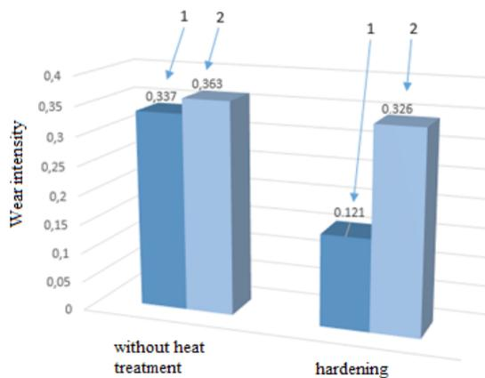
Pic. 7. Intensity of linear wear of samples without heat treatment and after laser hardening: 1 – wheel steel sample; 2 – rail steel counterbody [14].
