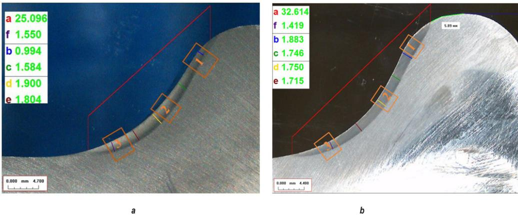
**Pic. 4. Macrostructure of the sample cut out from the wheel tyre:**
