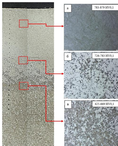
*Pic. 6. Microstructure and microhardness of various areas of the hardened section 2 after laser hardening [developed and compiled by the authors].*
