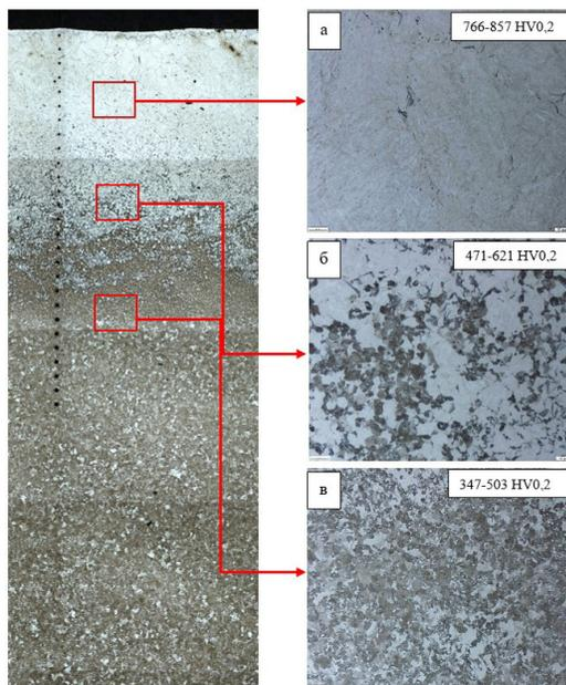
*Pic. 5. Microstructure and microhardness of various areas of the hardened section 2 after plasma hardening.*
