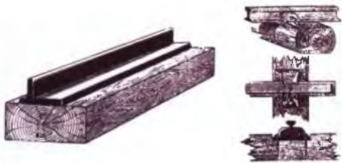
Pic. 2. Image of a wooden bench with an iron plate with a rim (corner rail). [Electronic resource]: http://www.rzd-expo.ru/history/history_of_railway_track/ . Last accessed 11.06.2021.
