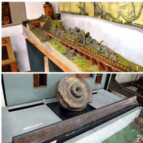
Pic. 7. Pig-iron horse-drawn road in Zmeinogorsk: 1 – model of the «chugunka»; 2 – a fragment of a cast-iron rail and a bogie wheel. Zmeinogorsk «chugunka» – progenitor of Russian railways // https://chuguntv.ru . [Electronic resource]: https://chuguntv.ru/zmeinogorskaya-chugunka-prarodite . Last accessed 11.06.2021.
