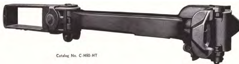
Pic. 5. AAR (H) type automatic coupler with yoke [16].
