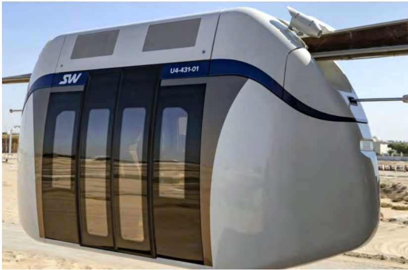
Pic. 11. Passenger car of A. E. Yunitskiy's system SkyWay [Unicar vehicle U4-431. Operation manual. Minsk, Strunnye technology LLC., 2018, P. 220].
