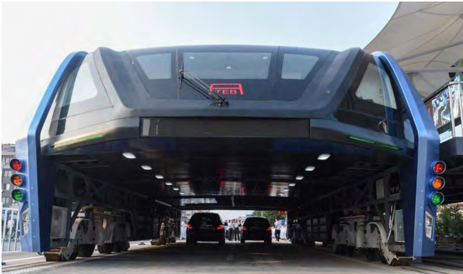
Pic. 4. A bus moving in the general flow over passenger cars (in Russian). [Electronic resource]: https://www.kommersant.ru/gallery/3054311#id1307215 . Last accessed 12.01.2022.
