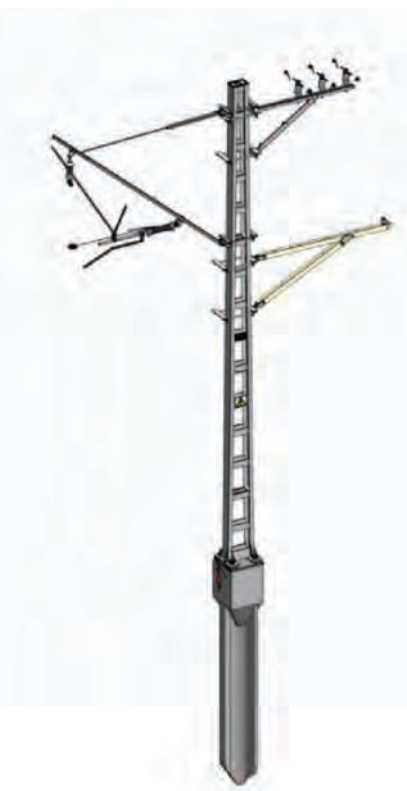
Pic. 3. An example of assembling a complex family. Catenary pole [developed by the authors].
