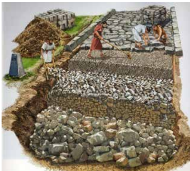
Pic. 5. Artistic illustration of the technology of building Roman roads with layer-by-layer detailing of masonry (How Roman roads were built. [Electronic resource]: https://pikabu.ru/story/kak_stroilis_rimskie_dorogi_5870592 . Last accessed 11.06.2021).
