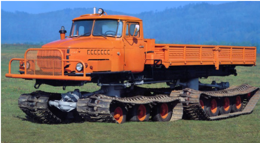
Pic. 5. Ural-5920 eracked all-terrain vehicle.
