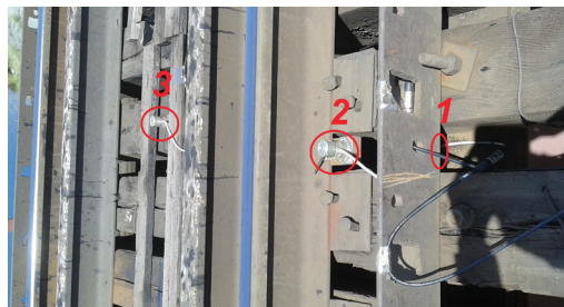
Pic. 2. General view of a metal superstructure with vibration sensors located on elements: 1 – middle of a beam span structure; 2 – rail base; 3 – middle of a sleeper.
