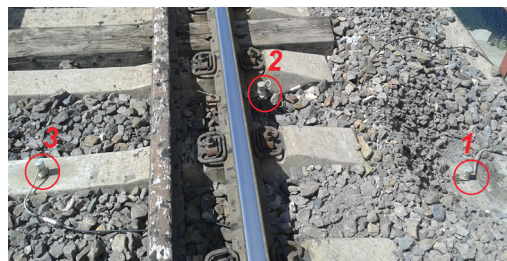
Pic. 4. General view of a concrete span with vibration sensors located on elements: 1 – middle of a beam span structure; 2 – rail base; 3 – middle of a sleeper.
