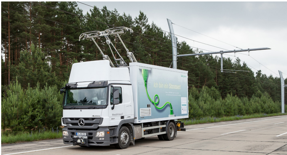
Pic. 5. Electric-powered system for heavy good vehicles on a specially built test track in the north of Berlin, Germany. (Photo: Siemens. https://press.assets.siemens.com/content/siemens/press/ui/en/search.htm#/asset/sid:320d002d-fa74-4a64-882c-715abfa3b6e5 ).
