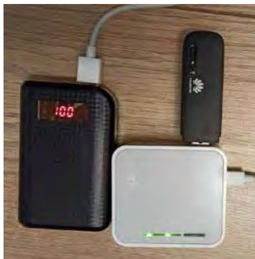
Pic. 2. Image of Wi-Fi scanner No. 2: TP-LINK assembled.
